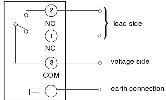
Fig. 2. C6058 connection diagram
