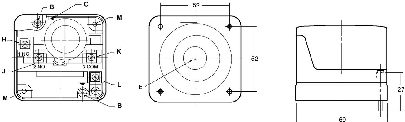
A Bracket mounting hole (3), M4 tapping, depth 5 mm
