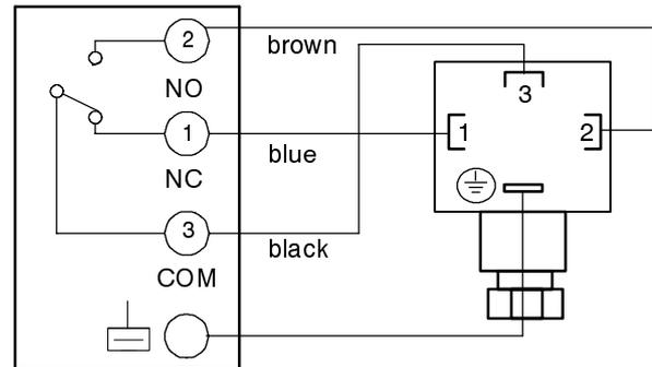
Fig. 3. C6058 connection diagram with DIN plug
